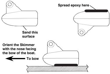
Epoxy transducer to hull.
